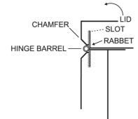
LIDSLOTRABBETInternational and the lid and body. The chamfer should end approx-<br/>imately ¾4" in front of the slot in order to accommodate a rabbet that also needs to be cut. The purpose of the rabbet cut is to allow the box lid to sit flat on the body. A straight bit can be used to cut the rabbet.
