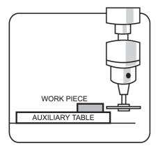
If you assemble your box body and lid before cutting your hinge slots, you will need to create a simple right angle carriage jig that supports your box lid and body as you cut your slots. Again, stops can be used to limit the depth of your hinge slots.
